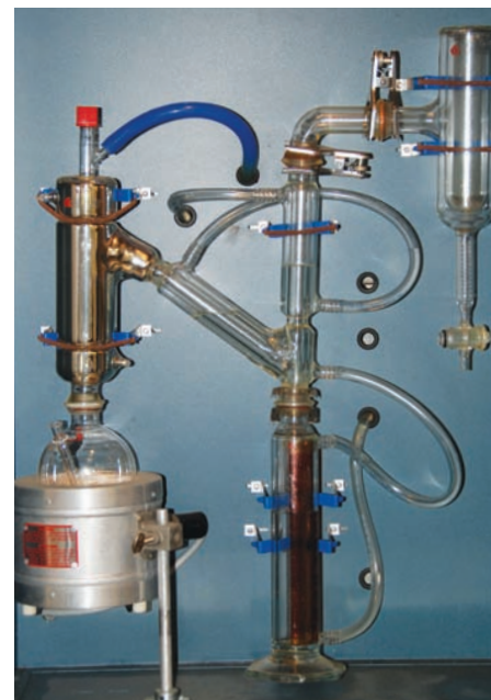
Vacuum Distillation apparatus for Testing Biodiesels Standards
