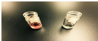
Figure 4: Comparison of QuEChERS extracts before and after dSPE cleanup (from left to right: hard candies and gummies)
