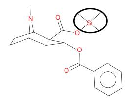
**Figure 1.** Trimethylsilyl derivative of benzoylecgonine. The underivatized compound has a carboxyl group and is too polar to pass through a GC column.
