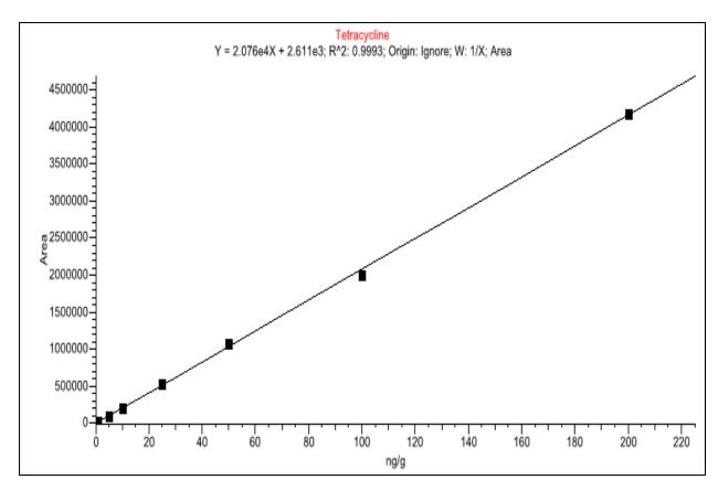
**Figure 2.** Example of an eight-point matrix-matched calibration curve (0.5-200  $\mu$ g/kg, equivalent to 2.5-1000 ng/mL in final extract).
